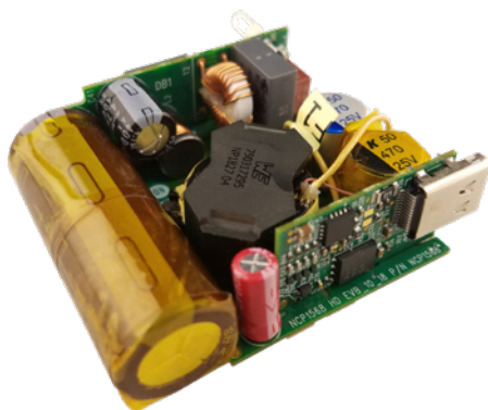
Ultra-high Density 60-W USB PD Adapter using the NCP1568 ACF Controller
