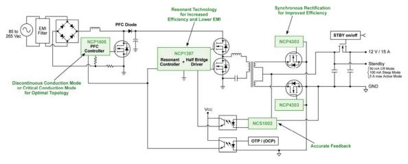
All-in-One Power Supply Simplified Block Diagram
