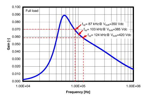
Figure 4: Gain Characteristics
