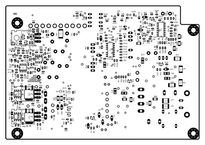
Figure 15: Bottom side components
