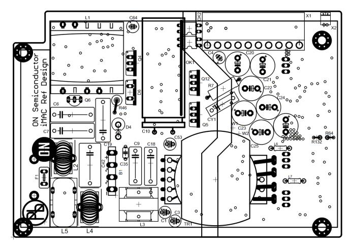
Figure 13: Top side components
