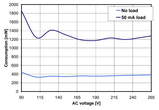
Figure 9: Light load efficiency measurements
