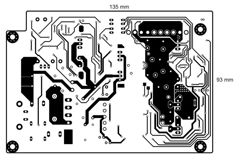
Figure 12: PCB top side
