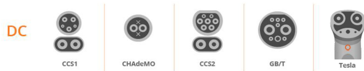
Figure 7. Fast DC Charger Connector Types. Tesla uses a proprietary connector in North America and other regions. In Europe and other regions where CCS and CHAdeMO networks are deployed, Tesla is adapting to these systems. Source: EnelX
