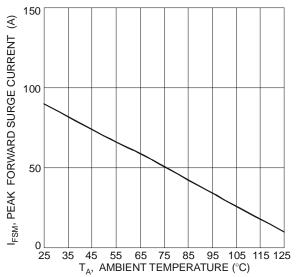
Fig. 8 Non-Repetitive Forward Surge Current Derating Curve
