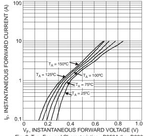
Fig. 2 Typ. Forward Characteristics - B350A thru B360A
