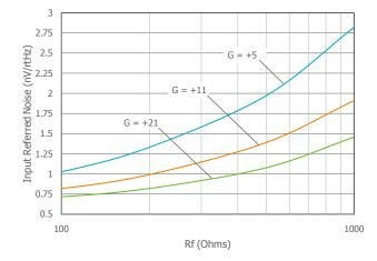
Figure 3: Input Referred Voltage Noise vs. Rf and Rq
