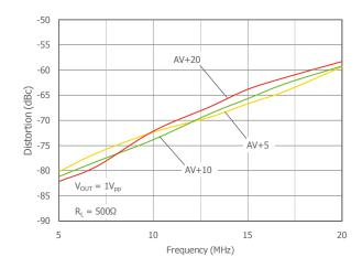
$T_A = 25$ °C,  $V_S = \pm 5$ V,  $R_f = 100\Omega$ ,  $R_L = 500\Omega$ , G = 5; unless otherwise noted.
