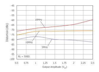
2nd Harmonic Distortion vs. Gain at  $V_S = 5V$
