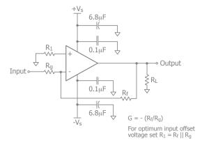
Figure 2. Typical Inverting Gain Circuit
