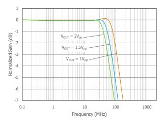
Inverting Frequency Response at  $V_S = 5V$
