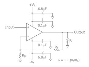
Figure 1. Typical Non-Inverting Gain Circuit
