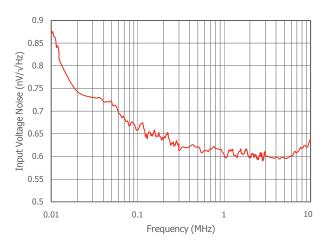
$T_A=25^{\circ}\text{C},\,V_S=\pm5\text{V},\,R_f=100\Omega,\,R_L=500\Omega$  , G=5; unless otherwise noted.
