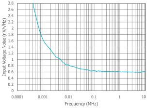
Input Voltage Noise (>10kHz)
