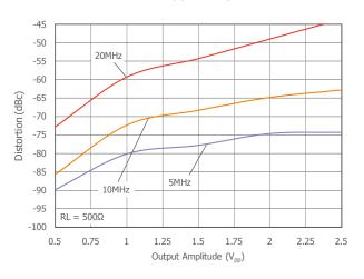
3rd Harmonic Distortion vs. Gain Freq at  $V_S = 5V$
