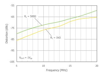
3rd Harmonic Distortion vs.  $V_{OUT}$  at  $V_S = 5V$
