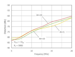
$T_A=25^{\circ}\text{C},\,V_S=\pm5\text{V},\,R_f=100\Omega,\,R_L=500\Omega$  , G=5; unless otherwise noted.
