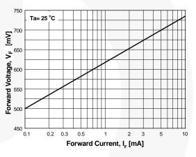
Figure 4. Forward Voltage vs. Forward Current  $V_{\text{F}}$  - 0.1 to 10 mA
