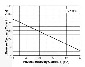
Figure 8. Reverse Recovery Time vs. Reverse Recovery Current
