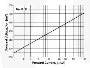
Figure 3. Forward Voltage vs. Forward Current  $\mbox{\sc V}_{\mbox{\sc F}}$  - 1 to 100  $\mbox{\sc {\sc H}}\mbox{\sc A}$
