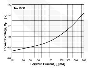
Figure 5. Forward Voltage vs. Forward Current  $V_{\text{F}}$  - 10 to 800 mA
