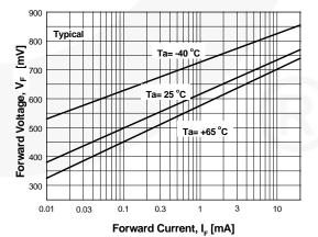
Figure 6. Forward Voltage vs. Ambient Temperature  $V_F$  - 0.01 - 20 mA (-40 to +65  $^{\circ}\text{C})$
