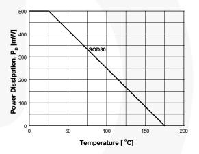
Figure 10. Power Derating Curve
