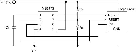
Notes: • Vs detection voltage can be adjusted externally.
