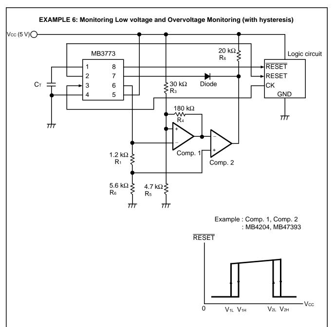
Notes: • Comp. 1 and Comp. 2 are used to monitor for overvoltage while the MB3773 is used to monitor for low voltage. Detection voltages V<sub>1</sub>L/V<sub>1</sub>H at the time of low voltage are approximately 4.2 V/4.3 V. Detection voltages V<sub>2</sub>L/V<sub>2</sub>H at the time of overvoltage are approximately 6.0 V/6.1 V. For the formulas for finding hysteresis width and detection voltage, see EXAMPLE 4.
