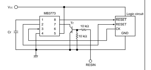
Note : Feeding the signal to terminal RESIN and turning on Tr sets the  $\overline{\text{RESET}}$  terminal to Low and the RESET terminal to High.
