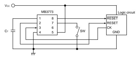
Note: Grounding pin 7 at the time of SW ON sets RESET (pin 8) to Low and RESET (pin 2) to High.
