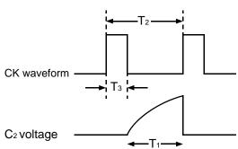
Example: Setting C and R allow the upper T<sub>1</sub> value to be set (Refer to the table below).
