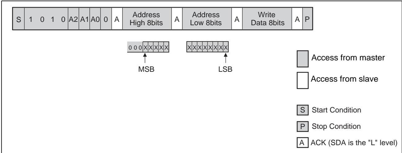
Note : In the MB85RC64V, input "000" to the upper 3 bits of the MSB because the address is expressed with 13 bits.
