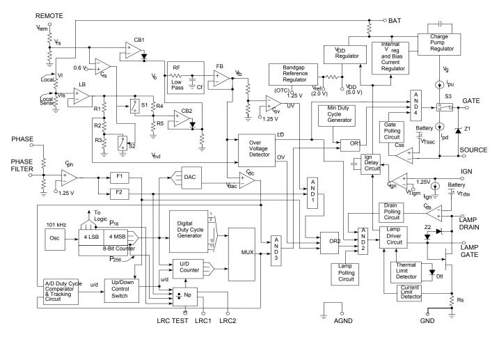
Figure 1. 33099 Simplified Internal Block Diagram
