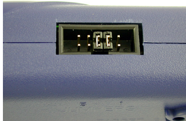
Figure 2-10: Jumper Settings for Target Power Connection via Cyclone PRO Board Power and Power Out Jack of Cyclone PRO
