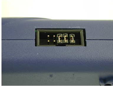
Figure 2-12: Jumper Settings for Target Power Connection via Cyclone PRO Board Power and Pin 15 of Cyclone PRO MON08 Connector
