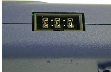
Figure 2-16: Jumper Settings For Power IN Jack And MON08 Header Pin 15
