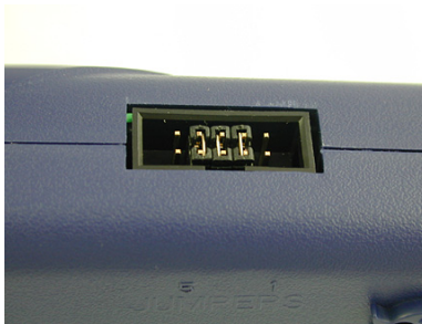
Figure 2-14: Jumper Settings for Target Power Connection via Cyclone PRO Board Power and Pin 6 of Cyclone PRO BDM Connector
