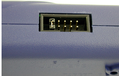
Figure 2-8: Jumper Settings for Target Power Connection via Power In and Power Out Jacks Of Cyclone PRO
