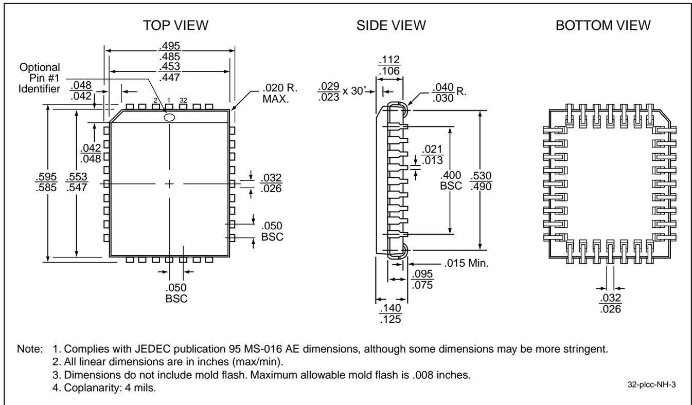
**32-LEAD PLASTIC LEAD CHIP CARRIER (PLCC)**
