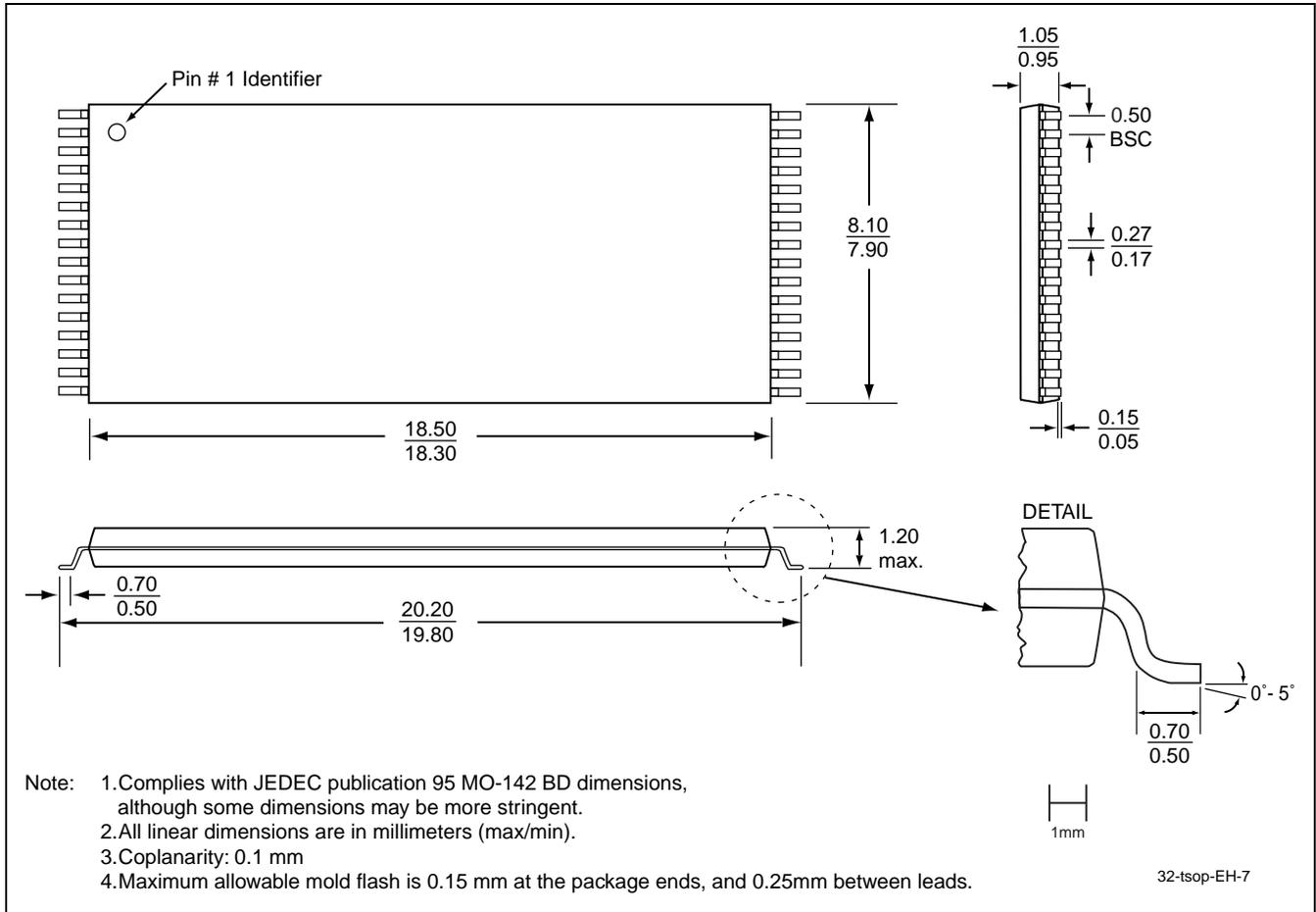
**32-LEAD THIN SMALL OUTLINE PACKAGE (TSOP) 8MM X 20MM**
