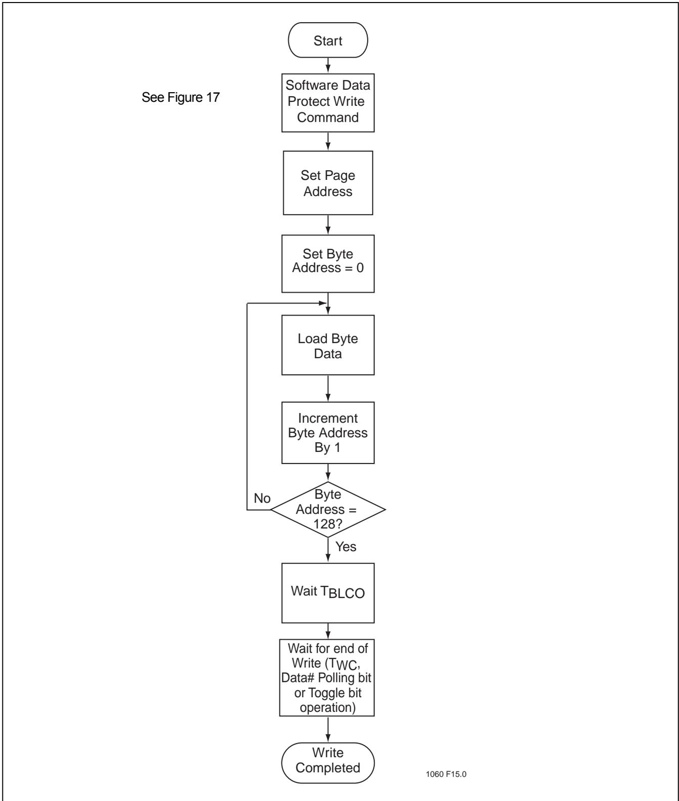
FIGURE 15: WRITE ALGORITHM
