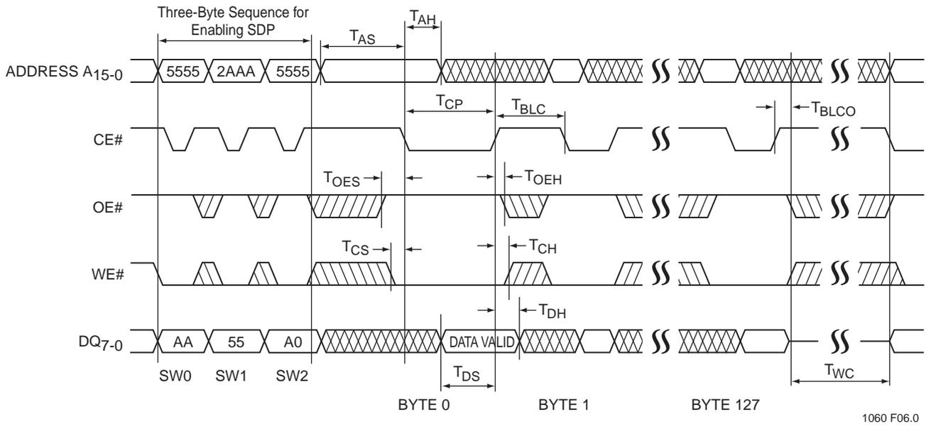
**FIGURE 6: CE# CONTROLLED PAGE-WRITE CYCLE TIMING DIAGRAM**
