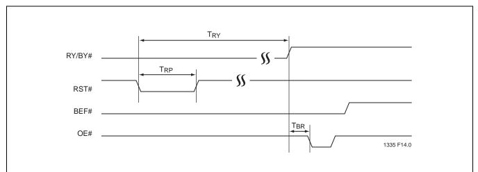
FIGURE 19: RST# Timing (during Sector- or Block-Erase operation)
