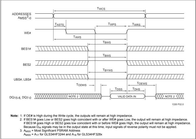
FIGURE 5: PSRAM Write Cycle Timing Diagram (WE# Controlled)<sup>1</sup>
