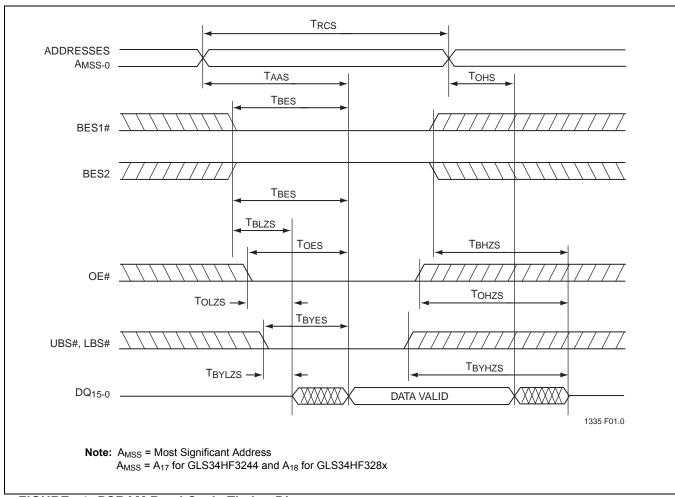
FIGURE 4: PSRAM Read Cycle Timing Diagram
