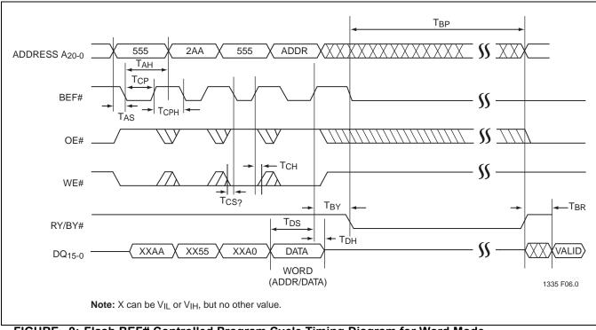
FIGURE 9: Flash BEF# Controlled Program Cycle Timing Diagram for Word Mode (For Byte Mode A<sub>-1</sub> = Address Input)
