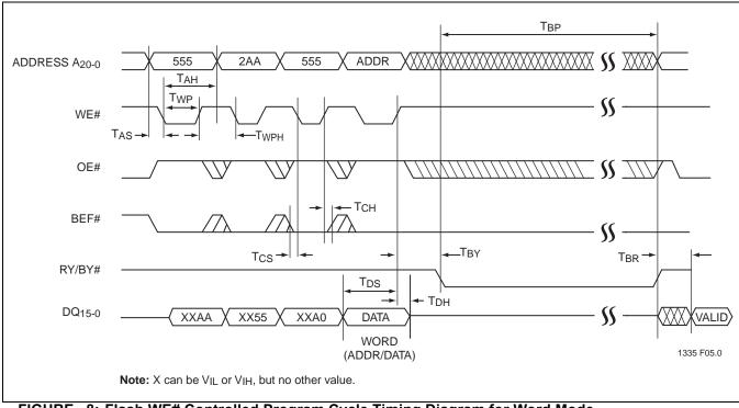
FIGURE 8: Flash WE# Controlled Program Cycle Timing Diagram for Word Mode (For Byte Mode A<sub>-1</sub> = Address Input)
