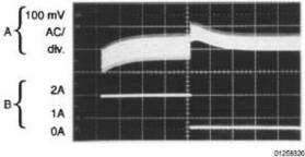
Horizontal Time Base: 200 µs/div. A: Output Voltage, 100 mV/div. (AC)
