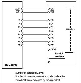
Figure 9 Parallel bus configuration
