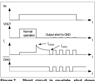
Figure 7 Short circuit in on-state, shut down down by overtemperature, restart by cooling
