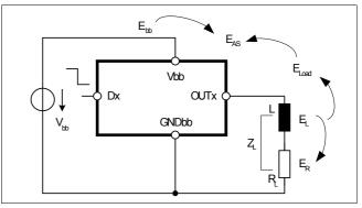
Figure 4 Inductive load switch-off energy dissipation (each channel)
