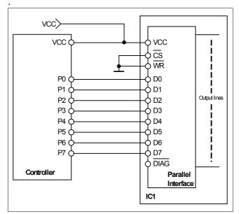
Figure 10 Parallel Direct Control
