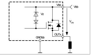
Figure 3 Inductive and overvoltage output clamp (each channel)
