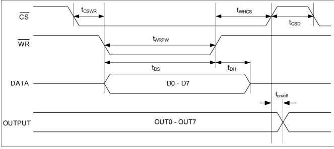
Figure 11 Parallel input - output timing diagram
