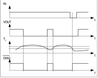
Figure 5 Overtemperature detection
