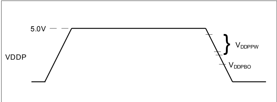
Figure 8 Supply Threshold Parameters
