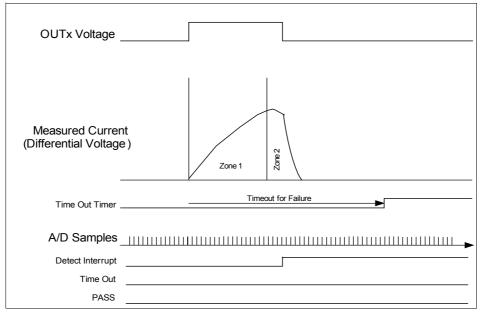
Figure 18 Current Profile Diagram - Detection Interrupted Failure
