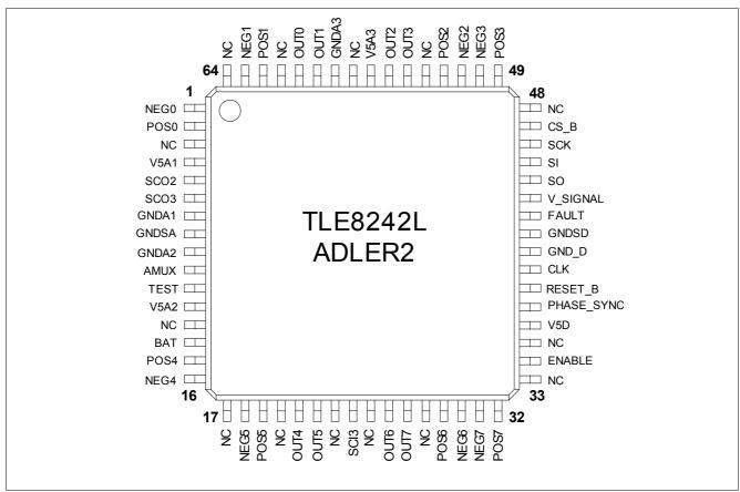
Figure 6 Pin Configuration
