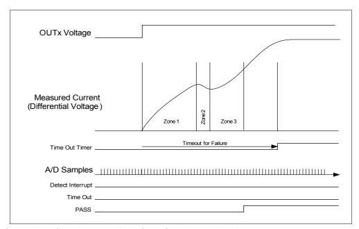
Figure 15 Current Profile Diagram - Waveform Showing Valve Movement
