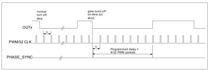
Figure 8 Phase Synchronization Diagram
