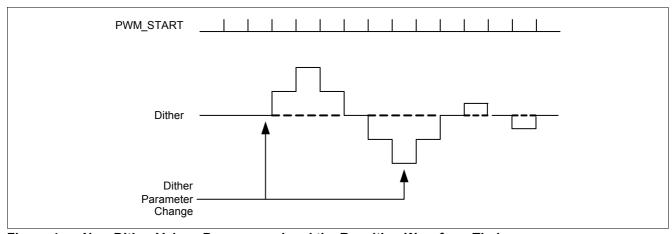
Figure 4 New Dither Values Programmed and the Resulting Waveform Timing
