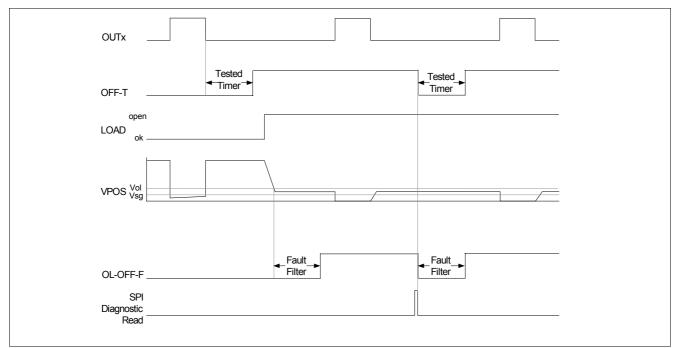
Figure 13 Off-State Diagnostics Timing Diagram - open
