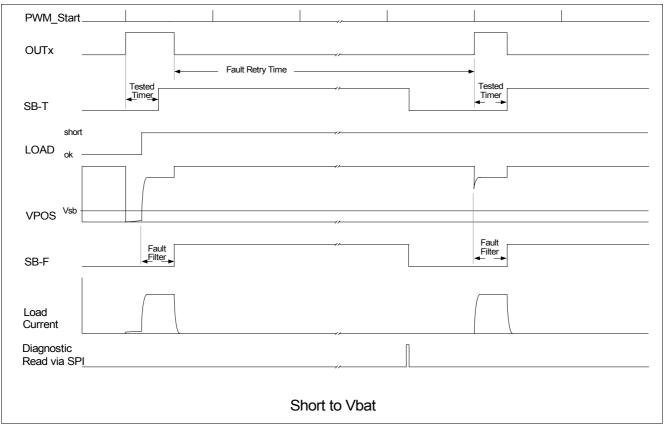
Figure 10 On-State Diagnostic Timing - Short to Vbat
