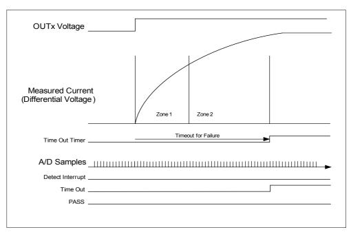
Figure 17 Current Profile Diagram - Time Out Failure
