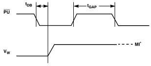
\*MI in the AC timing diagram refers to the minimum incremental change in the wiper voltage.
