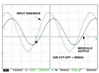
FIGURE 12. FREQUENCY RESPONSE (500kHz)
