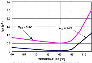
FIGURE 2. STANDBY I<sub>CC</sub> vs TEMPERATURE
