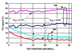
FIGURE 10. TC FOR VOLTAGE DIVIDER MODE IN ppm
