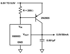
FIGURE 36. PRECISION 5V, 50mA REFERENCE
