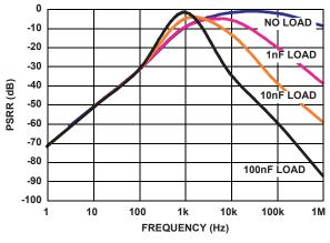
FIGURE 10. PSRR vs CAP LOAD
