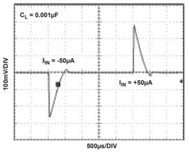
FIGURE 24. 50µA LOAD TRANSIENT RESPONSE
