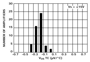
FIGURE 15. OFFSET VOLTAGE DRIFT DISTRIBUTION,  $V_S = \pm 15V$
