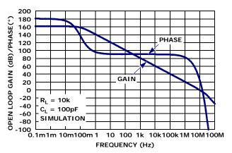
FIGURE 26. OPEN-LOOP GAIN, PHASE vs FREQUENCY,  $\mathbf{R_{I}=10k}\Omega,\,\mathbf{C_{I}=100pF}$
