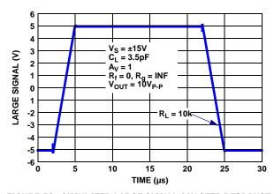
FIGURE 53. SIMULATED LARGE SIGNAL 10V STEP RESPONSE
