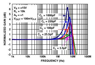
FIGURE 50. CHARACTERIZED CLOSED LOOP GAIN vs CL
