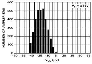
FIGURE 13. INPUT OFFSET VOLTAGE DISTRIBUTION,  $V_S = \pm 15V$
