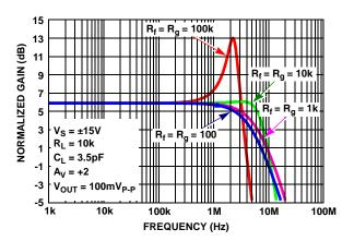
FIGURE 47. SIMULATED CLOSED LOOP GAIN vs  $\rm R_{\it f}/R_{\it g}$
