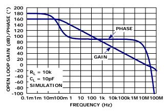
FIGURE 25. OPEN-LOOP GAIN, PHASE vs FREQUENCY,  $\mathbf{R_L=10k}\Omega,\,\mathbf{C_L=10pF}$
