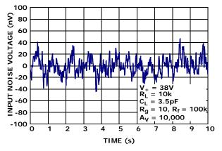
FIGURE 3. INPUT NOISE VOLTAGE 0.1Hz to 10Hz
