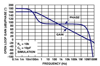
FIGURE 54. SIMULATED OPEN-LOOP GAIN, PHASE vs FREQUENCY
