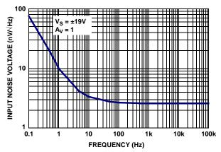
FIGURE 42. CHARACTERIZED INPUT NOISE VOLTAGE
