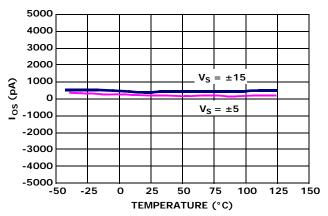
FIGURE 11.  $I_{OS}$  vs TEMPERATURE vs SUPPLY VOLTAGE
