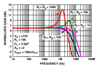
FIGURE 46. CHARACTERIZED CLOSED LOOP GAIN vs  $R_f/R_g$
