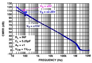
FIGURE 56. CHARACTERIZED CMRR vs FREQUENCY
