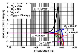
FIGURE 51. SIMULATED CLOSED LOOP GAIN vs CL
