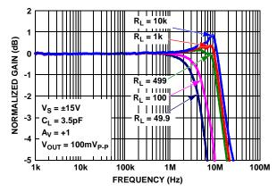
FIGURE 48. CHARACTERIZED CLOSED LOOP GAIN vs  $\rm R_L$
