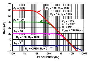
FIGURE 44. CHARACTERIZED CLOSED LOOP GAIN vs FREQUENCY
