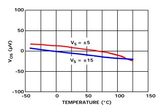
FIGURE 8.  $V_{OS}$  vs TEMPERATURE vs  $V_{SUPPLY}$
