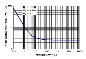
FIGURE 2. INPUT NOISE VOLTAGE SPECTRAL DENSITY
