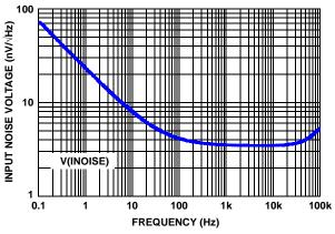
FIGURE 43. SIMULATED INPUT NOISE VOLTAGE
