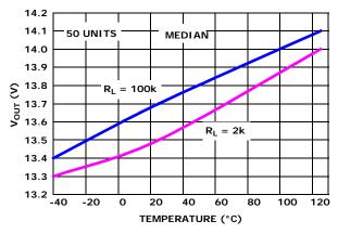
FIGURE 23.  $V_{OH}$  vs TEMPERATURE,  $V_{S} = \pm 15V$
