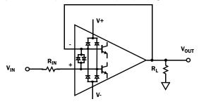
FIGURE 38. INPUT ESD DIODE CURRENT LIMITING- UNITY GAIN
