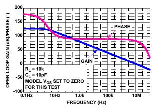
FIGURE 55. SIMULATED OPEN-LOOP GAIN, PHASE vs FREQUENCY
