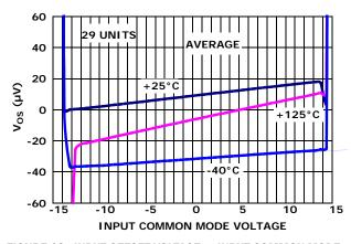
FIGURE 12. INPUT OFFSET VOLTAGE vs INPUT COMMON MODE VOLTAGE,  $V_S = \pm 15V$
