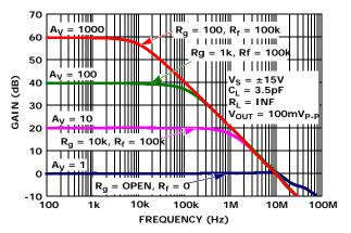
FIGURE 27. FREQUENCY RESPONSE vs CLOSED LOOP GAIN
