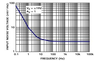
FIGURE 4. INPUT NOISE VOLTAGE SPECTRAL DENSITY
