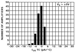
FIGURE 22. INPUT OFFSET CURRENT DISTRIBUTION,  $V_S = \pm 5V$
