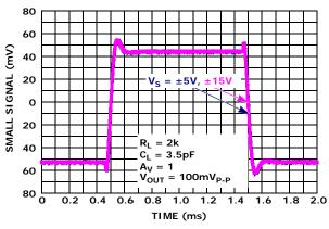
FIGURE 34. SMALL SIGNAL TRANSIENT RESPONSE,  $V_S = \pm 5V$ ,  $\pm 15V$
