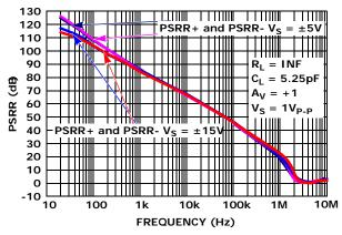
FIGURE 6. PSRR vs FREQUENCY,  $V_S = \pm 5V$ ,  $\pm 15V$
