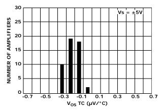
FIGURE 16. OFFSET VOLTAGE DRIFT DISTRIBUTION,  $V_S = \pm 5V$
