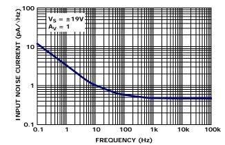
FIGURE 5. INPUT NOISE CURRENT SPECTRAL DENSITY
