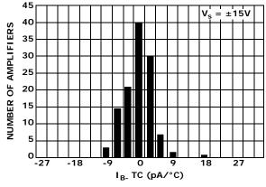
FIGURE 19. IB. INPUT BIAS CURRENT DRIFT DISTRIBUTION,  $V_S = \pm 15 \text{V} \label{eq:VS}$
