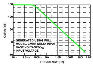
FIGURE 57. SIMULATED CMRR vs FREQUENCY
