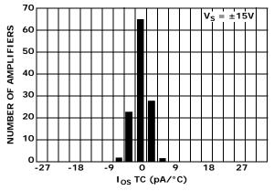
FIGURE 21. INPUT OFFSET CURRENT DISTRIBUTION,  $V_S = \pm 15V$
