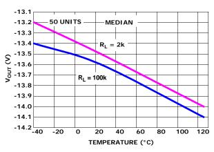
FIGURE 24.  $V_{OL}$  vs TEMPERATURE,  $V_{S} = \pm 15V$
