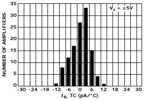
FIGURE 20. IB- INPUT BIAS CURRENT DRIFT DISTRIBUTION,  $V_S = \pm 5 \text{V} \label{eq:VS}$
