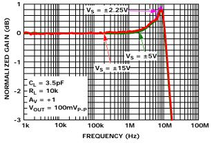
FIGURE 31. GAIN vs FREQUENCY vs SUPPLY VOLTAGE
