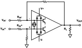
FIGURE 39. INPUT ESD DIODE CURRENT LIMITING DIFFERENTIAL INPUT
