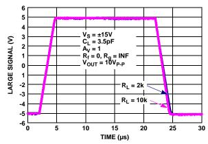
FIGURE 52. CHARACTERIZED LARGE SIGNAL 10V STEP RESPONSE
