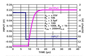
FIGURE 36. NEGATIVE OUTPUT OVERLOAD RESPONSE TIME,  $V_S$ = ±15V
