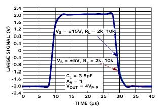
FIGURE 33. LARGE SIGNAL TRANSIENT RESPONSE vs  $R_L V_S = \pm 5V, \pm 15V$
