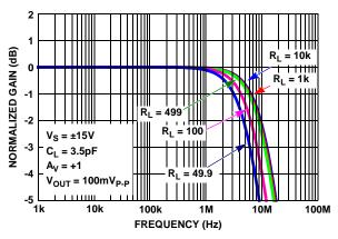
FIGURE 49. SIMULATED CLOSED LOOP GAIN vs R<sub>L</sub>
