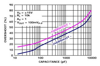
FIGURE 37. % OVERSHOOT vs LOAD CAPACITANCE,  $V_S = \pm 15V$
