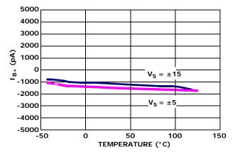
FIGURE 9. IB+ vs TEMPERATURE vs SUPPLY VOLTAGE
