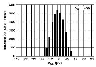
FIGURE 14. INPUT OFFSET VOLTAGE DISTRIBUTION,  $V_S = \pm 5V$
