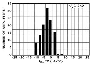
FIGURE 18.  $I_{B+}$  INPUT BIAS CURRENT DRIFT DISTRIBUTION,  $V_S = \pm 5 \text{V}$
