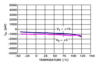
FIGURE 10. IB- vs TEMPERATURE vs SUPPLY VOLTAGE
