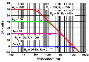
FIGURE 45. SIMULATED CLOSED LOOP GAIN vs FREQUENCY
