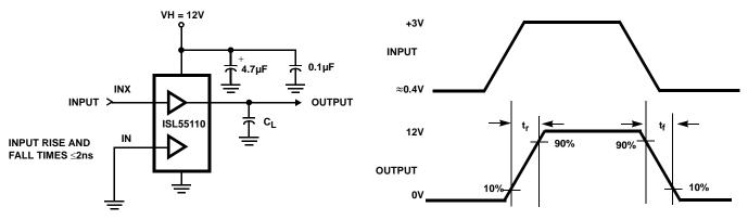
FIGURE 1. TEST CIRCUIT RISE (t\_R)/FALL(t\_F) THRESHOLDS
