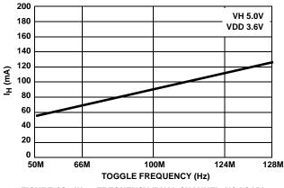
FIGURE 12. IH vs FREQUENCY (DUAL CHANNEL, NO LOAD)
