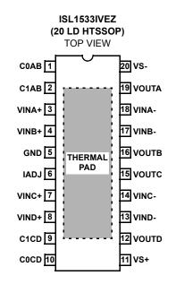
THERMAL PAD TO BE CONNECTED TO GND
