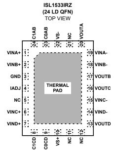
THERMAL PAD TO BE CONNECTED TO GND
