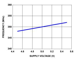
FIGURE 11. FREQUENCY vs SUPPLY VOLTAGE
