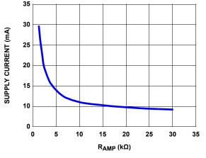
FIGURE 10. SUPPLY CURRENT vs RAMP
