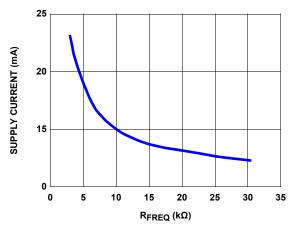
FIGURE 9. SUPPLY CURRENT vs RFREQ
