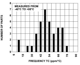
FIGURE 4. FREQUENCY DRIFT WITH TEMPERATURE
