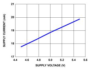
FIGURE 13. SUPPLY CURRENT vs SUPPLY VOLTAGE
