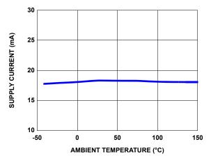
FIGURE 16. SUPPLY CURRENT vs TEMPERATURE
