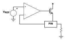
FIGURE 21. RAMP AND RFREQ PIN INTERFACE
