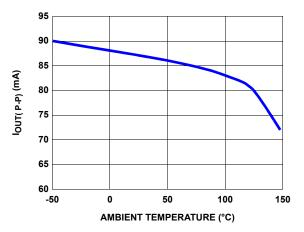
FIGURE 15. PEAK-TO-PEAK OUTPUT CURRENT vs TEMPERATURE
