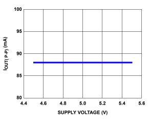
FIGURE 12. PEAK-TO-PEAK OUTPUT CURRENT vs SUPPLY VOLTAGE
