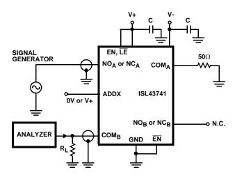
FIGURE 7. CROSSTALK TEST CIRCUIT
