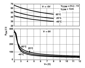
FIGURE 10. ON RESISTANCE vs SUPPLY VOLTAGE
