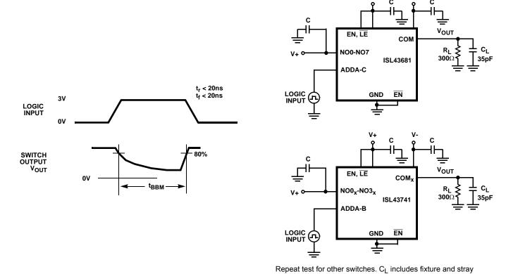
FIGURE 3A. t<sub>BBM</sub> MEASUREMENT POINTS
