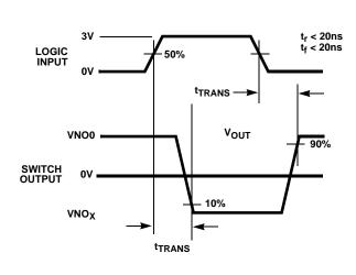
Logic input waveform is inverted for switches that have the opposite logic sense.
