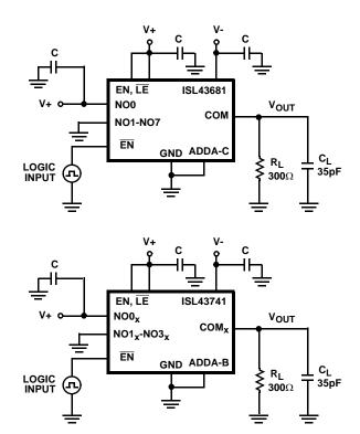
Repeat test for other switches. C<sub>L</sub> includes fixture and stray capacitance.
