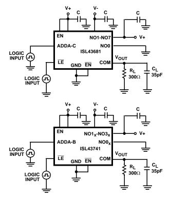
Logic input waveform is inverted for switches that have the opposite logic sense.
