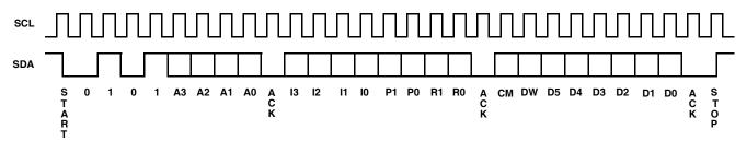
FIGURE 4. THREE-BYTE INSTRUCTION SEQUENCE
