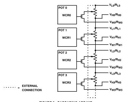
FIGURE 9. CASCADING ARRAYS
