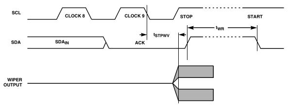
FIGURE 13. WRITE CYCLE AND WIPER RESPONSE TIMING
