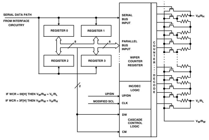
FIGURE 8. DETAILED POTENTIOMETER BLOCK DIAGRAM
