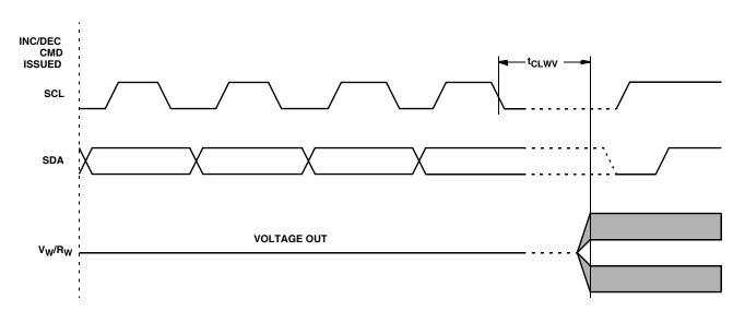
FIGURE 6. INCREMENT/DECREMENT TIMING LIMITS
