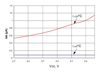
FIGURE 2. STANDBY I<sub>CC</sub> vs V<sub>CC</sub>
