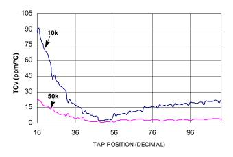
FIGURE 8. TC FOR VOLTAGE DIVIDER MODE IN ppm
