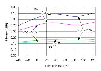
FIGURE 5. ZSerror vs TEMPERATURE
