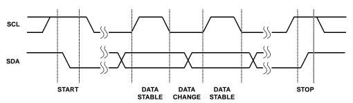
FIGURE 12. VALID DATA CHANGES, START AND STOP CONDITIONS
