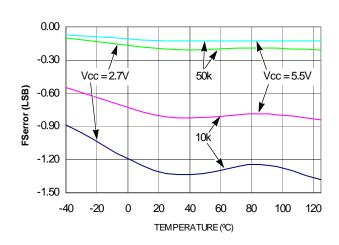
FIGURE 6. FSerror vs TEMPERATURE
