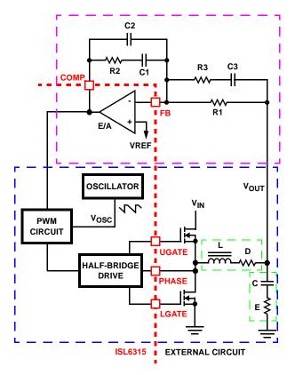
FIGURE 8. VOLTAGE-MODE BUCK CONVERTER COMPENSATION DESIGN
