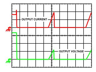
FIGURE 4. OVERCURRENT BEHAVIOR IN HICCUP MODE
