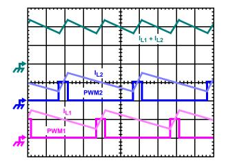
FIGURE 2. PWM AND INDUCTOR-CURRENT WAVEFORMS **FOR 2-PHASE CONVERTER**
