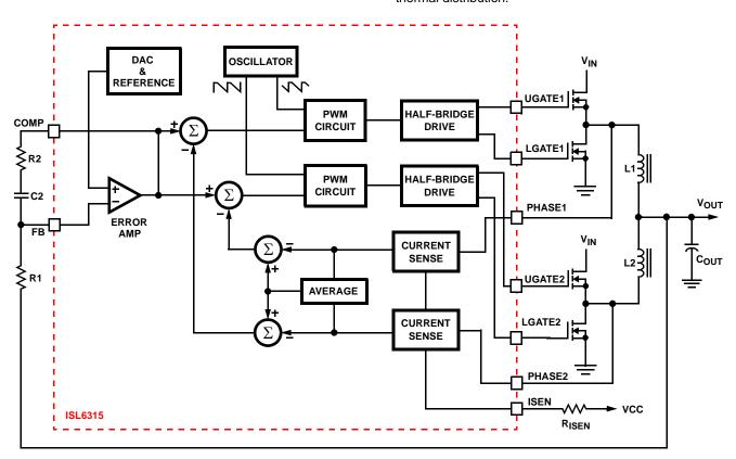
FIGURE 1. SIMPLIFIED BLOCK DIAGRAM OF THE ISL6315 VOLTAGE AND CURRENT FEEDBACK
