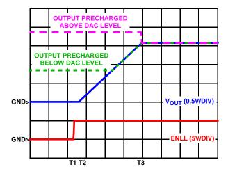
FIGURE 7. SOFT-START WAVEFORMS FOR ISL6315-BASED MULTIPHASE CONVERTER
