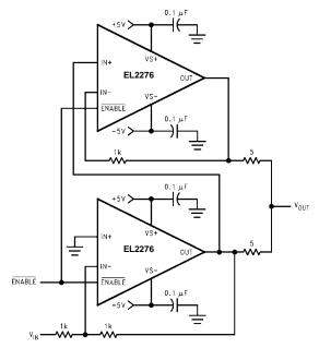
INVERTING 200mA OUTPUT CURRENT DISTRIBUTION AMPLIFIER
