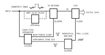
Horizontal genlock provides clock for an analog to digital converter, digitizing analog video.
