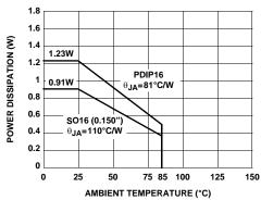
Package Power Dissipation vs Ambient Temperature JEDEC JESD51-7 High Effective Thermal Conductivity
