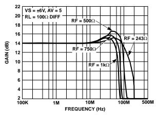
FIGURE 3. DIFFERENTIAL FREQUENCY RESPONSE WITH VARIOUS  $R_F$  (1/2 POWER MODE)
