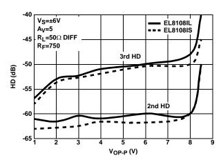
FIGURE 12. DISTORTION BETWEEN EL8108IL vs EL8108IS
