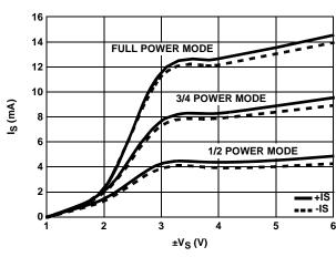
FIGURE 28. SUPPLY CURRENT vs SUPPLY VOLTAGE
