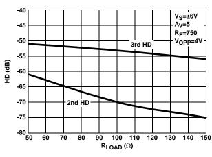
FIGURE 16. 2nd AND 3rd HARMONIC DISTORTION vs R<sub>LOAD</sub>
