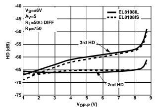
FIGURE 11. DISTORTION BETWEEN EL8108IL vs EL8108IS AT 5MHz
