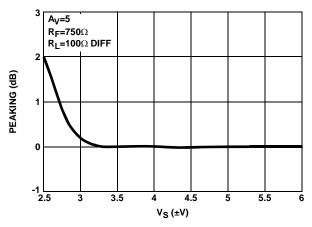
FIGURE 35. DIFFERENTIAL PEAKING vs SUPPLY VOLTAGE
