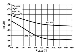
FIGURE 15. 2nd AND 3rd HARMONIC DISTORTION vs R<sub>LOAD</sub>
