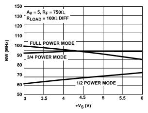
FIGURE 25. DIFFERENTIAL BANDWIDTH vs SUPPLY VOLTAGE
