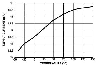
FIGURE 34. SUPPLY CURRENT vs TEMPERATURE
