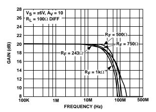
FIGURE 6. DIFFERENTIAL FREQUENCY RESPONSE WITH VARIOUS R<sub>F</sub> (1/2 POWER MODE)
