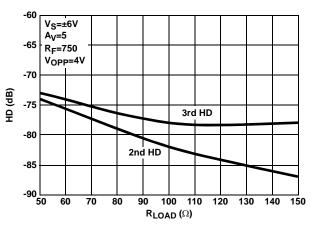
FIGURE 14. 2nd AND 3rd HARMONIC DISTORTION vs R<sub>LOAD</sub>
