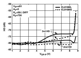
FIGURE 9. DISTORTION BETWEEN EL8108IL vs EL8108IS AT 2MHz
