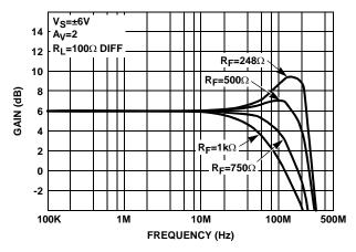
FIGURE 7. DIFFERENTIAL FREQUENCY RESPONSE WITH VARIOUS  $R_{\mathrm{F}}$
