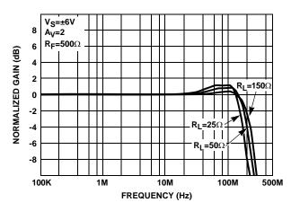
FIGURE 8. FREQUENCY RESPONSE FOR VARIOUS  $R_{\mbox{\scriptsize LOAD}}$
