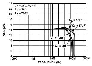
FIGURE 19. FREQUENCY RESPONSE WITH VARIOUS C<sub>L</sub>
