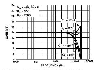
FIGURE 18. FREQUENCY RESPONSE vs VARIOUS C<sub>L</sub>
