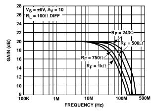
FIGURE 5. DIFFERENTIAL FREQUENCY RESPONSE WITH VARIOUS R<sub>F</sub> (3/4 POWER MODE)
