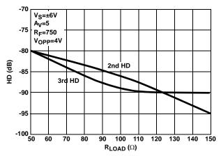
FIGURE 13. 2nd AND 3rd HARMONIC DISTORTION vs R<sub>LOAD</sub>
