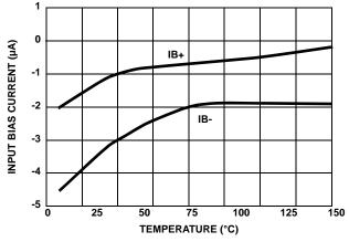
FIGURE 29. INPUT BIAS CURRENT vs TEMPERATURE
