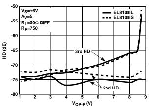
FIGURE 10. DISTORTION BETWEEN EL8108IL vs EL8108IS
