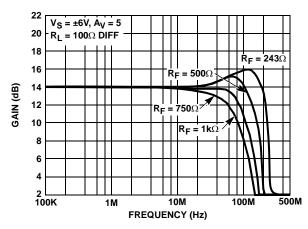
FIGURE 2. DIFFERENTIAL FREQUENCY RESPONSE WITH VARIOUS R<sub>F</sub> (3/4 POWER MODE)
