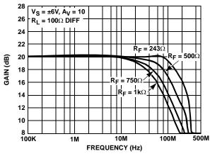
FIGURE 4. DIFFERENTIAL FREQUENCY RESPONSE WITH VARIOUS  $R_F$  (FULL POWER MODE)
