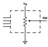
THREE TERMINAL POTENTIOMETER; VARIABLE VOLTAGE DIVIDER
