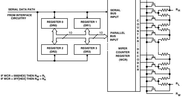
FIGURE 1. DETAILED POTENTIOMETER BLOCK DIAGRAM SERIAL INTERFACE DESCRIPTION
