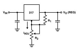
$V_{O}$  (REG) = 1.25V (1+R<sub>2</sub>/R<sub>1</sub>)+I<sub>adj</sub> R<sub>2</sub>
