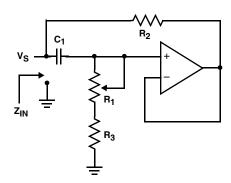
$Z_{IN} = R_2 + s R_2 (R_1 + R_3) C_1 = R_2 + s Leq$  $(R_1 + R_3) >> R_2$
