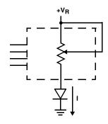
TWO TERMINAL VARIABLE RESISTOR; VARIABLE CURRENT
