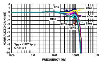
FIGURE 2. ISL59920 FREQUENCY RESPONSE (GAIN = 1)
