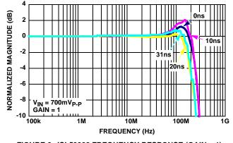
FIGURE 6. ISL59922 FREQUENCY RESPONSE (GAIN = 1)
