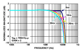
FIGURE 9. ISL59923 FREQUENCY RESPONSE (GAIN = 2)
