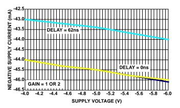
FIGURE 25. ISL59920  $I_{SUPPLY}$ - vs  $V_{SUPPLY}$ -
