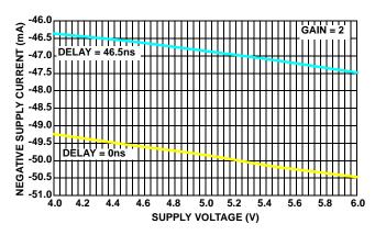
FIGURE 27. ISL59921 I<sub>SUPPLY</sub>- vs V<sub>SUPPLY</sub>-
