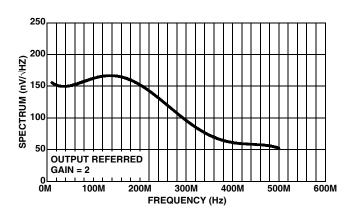
FIGURE 13. ISL59922 NOISE SPECTRUM (10k TO 500MHz)
