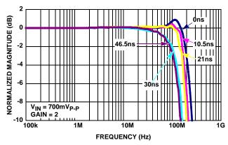
FIGURE 5. ISL59921 FREQUENCY RESPONSE (GAIN = 2)
