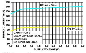
ISL59923  $I_{SUPPLY}$ + vs  $V_{SUPPLY}$ +
