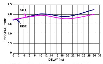
FIGURE 18. ISL59923 RISE/FALL TIME vs DELAY TIME (GAIN = 2)
