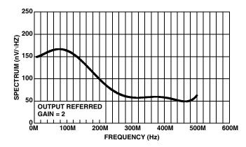
FIGURE 14. ISL59923 NOISE SPECTRUM (10k TO 500MHz)
