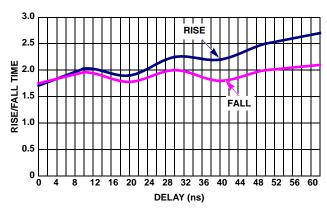
FIGURE 15. ISL59920 RISE/FALL TIME vs DELAY TIME (GAIN = 2)
