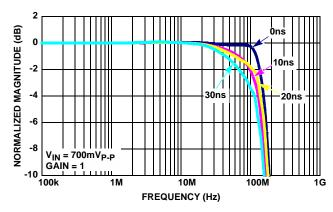
FIGURE 8. ISL59923 FREQUENCY RESPONSE (GAIN = 1)
