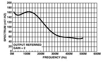
FIGURE 12. ISL59921 NOISE SPECTRUM (10k TO 500MHz)
