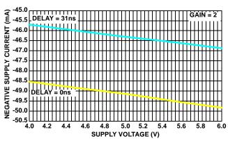
FIGURE 29. ISL59922 I<sub>SUPPLY</sub>- vs V<sub>SUPPLY</sub>-
