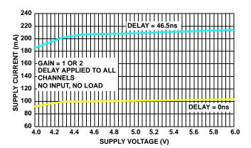
FIGURE 26. ISL59921 I<sub>SUPPLY</sub>+ vs V<sub>SUPPLY</sub>+
