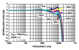
FIGURE 3. ISL59920 FREQUENCY RESPONSE (GAIN = 2)
