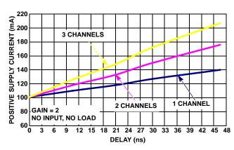
FIGURE 21. ISL59921 POSITIVE SUPPLY CURRENT ( $V_{SP}$ ) vs DELAY TIME
