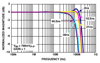
FIGURE 4. ISL59921 FREQUENCY RESPONSE (GAIN = 1)
