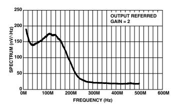
FIGURE 11. ISL59920 NOISE SPECTRUM (10k TO 500MHz)
