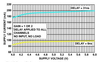
FIGURE 28. ISL59922 I<sub>SUPPLY</sub>+ vs V<sub>SUPPLY</sub>+
