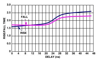
FIGURE 16. ISL59921 RISE/FALL TIME vs DELAY TIME (GAIN = 2)
