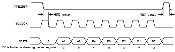
FIGURE 33. SERIAL TIMING
