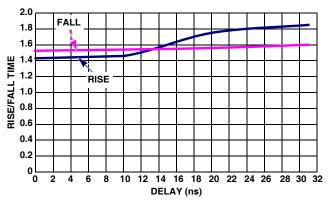
FIGURE 17. ISL59922 RISE/FALL TIME vs DELAY TIME (GAIN = 2)
