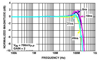
FIGURE 7. ISL59922 FREQUENCY RESPONSE (GAIN = 2)
