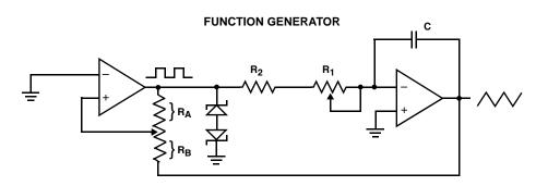
frequency  $\propto R_1, R_2, C$  amplitude  $\propto R_A, R_B$
