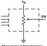
Three terminal Potentiometer; Variable voltage divider
