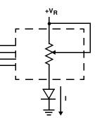
Two terminal Variable Resistor; Variable current
