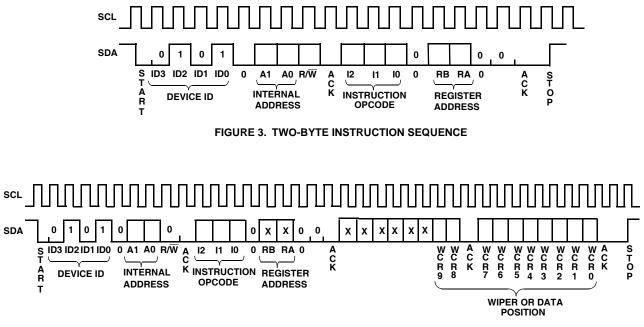
FIGURE 4. FOUR-BYTE INSTRUCTION SEQUENCE (WRITE OR READ FOR WCR OR DATA REGISTERS)
