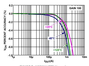
FIGURE 7. NORMALIZED  $V_{OA}$  vs  $I_{OUT}$
