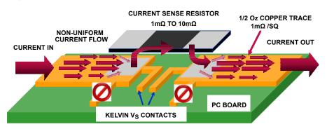
FIGURE 21. PC BOARD CURRENT SENSE KELVIN CONNECTION
