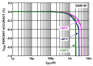
FIGURE 9. NORMALIZED  $V_{OA}$  vs  $I_{OUT}$
