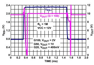
FIGURE 6.  $V_{OUT}$  vs  $V_{RS+}$ ,  $V_{SENSE} = 20$ mV TRANSIENT RESPONSE
