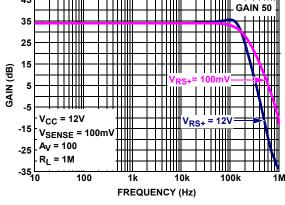
FIGURE 10. GAIN vs FREQUENCY  $V_{RS+}$ = 100mV/12V,  $V_{SENSE}$  = 100mV,  $V_{OUT}$  = 250mV<sub>P-P</sub>
