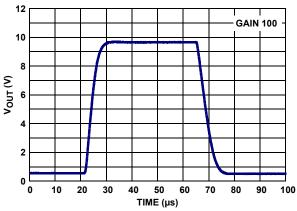
FIGURE 4. LARGE SIGNAL TRANSIENT RESPONSE  $V_{RS+} = 12V$ ,  $V_{SENSE} = 100 \text{mV}$
