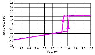
FIGURE 20. GAIN ACCURACY vs V<sub>RS+</sub> = 0V TO 2V
