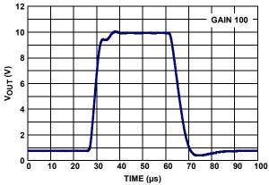
FIGURE 3. LARGE SIGNAL TRANSIENT RESPONSE  $V_{RS+} = 0.2V$ ,  $V_{SENSE} = 100 \text{mV}$
