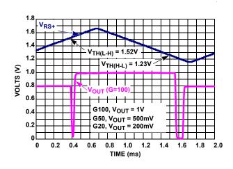
FIGURE 2. HIGH-SIDE AND LOW-SIDE THRESHOLD VOLTAGE
