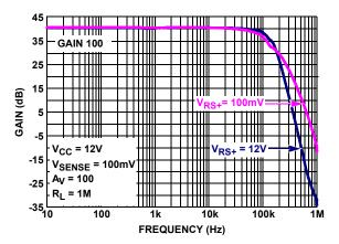
FIGURE 8. GAIN vs FREQUENCY  $V_{RS+}$ = 100mV/12V,  $V_{SENSE}$  = 100mV,  $V_{OUT}$  = 250mV<sub>P-P</sub>
