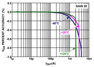
FIGURE 11. NORMALIZED  $V_{OA}$  vs  $I_{OUT}$
