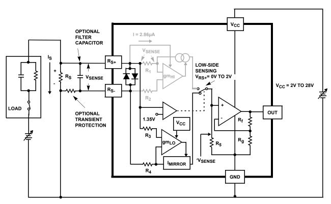
FIGURE 19. LOW-SIDE CURRENT DETECTION
