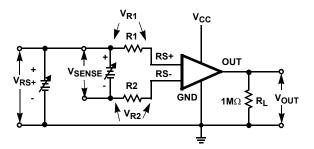
FIGURE 14. INPUT BIAS CURRENT, LEAKAGE CURRENT
