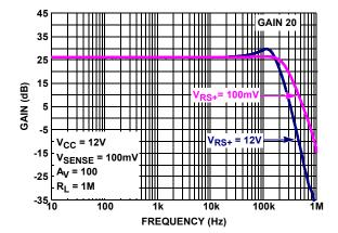
FIGURE 12. GAIN vs FREQUENCY  $V_{RS+}$ =100mV/12V,  $V_{SENSE}$  = 100mV,  $V_{OUT}$  = 250mV<sub>P-P</sub>
