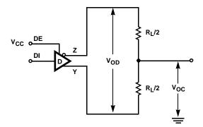
FIGURE 1A.  $V_{OD}$  AND  $V_{OC}$
