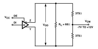
FIGURE 1B. VOD WITH COMMON MODE LOAD
