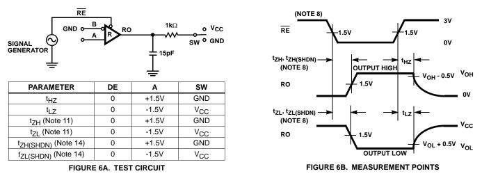
FIGURE 6. RECEIVER ENABLE AND DISABLE TIMES
