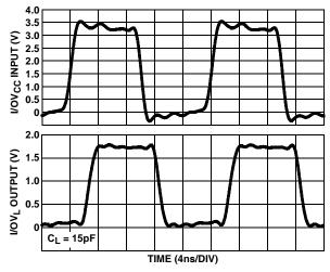
FIGURE 20. I/OVL OUTPUT WAVEFORMS (100Mbps)
