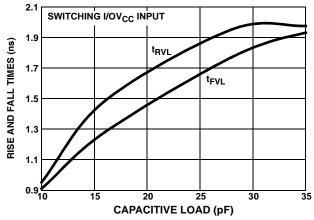
FIGURE 16. RISE/FALL TIME vs I/OVL CAPACITIVE LOAD
