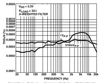
FIGURE 18. THD+N vs SIGNAL LEVELS vs FREQUENCY
