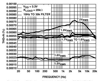
FIGURE 22. THD+N vs SIGNAL LEVELS vs FREQUENCY
