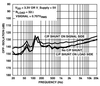
FIGURE 11. OFF-ISOLATION,  $0.707V_{\mbox{RMS}}$  SIGNAL,  $32\Omega$  LOAD
