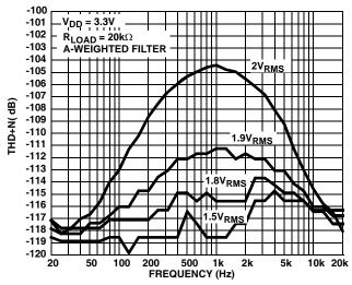
FIGURE 19. THD+N vs SIGNAL LEVELS vs FREQUENCY
