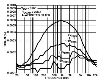
FIGURE 20. THD+N vs SIGNAL LEVELS vs FREQUENCY
