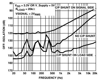
FIGURE 10. OFF-ISOLATION,  $2V_{RMS}$  SIGNAL,  $20k\Omega$ Load
