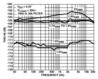
FIGURE 21. THD+N vs SIGNAL LEVELS vs FREQUENCY
