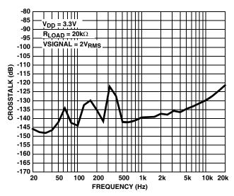
FIGURE 12. CHANNEL-TO-CHANNEL CROSSTALK
