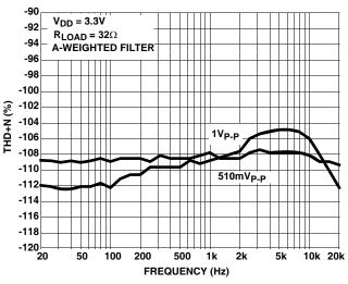
FIGURE 17. THD+N vs SIGNAL LEVELS vs FREQUENCY
