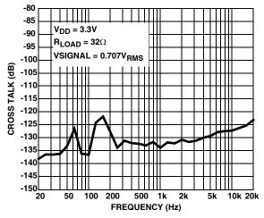
FIGURE 13. CHANNEL-TO-CHANNEL CROSSTALK
