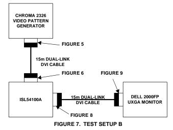
Given the input signal shown in Figure 6, the ISL54100A's TMDS output signal (Figure 8) is extremely clean. The output is an improvement over the original signal coming from the pattern generator in both amplitude and jitter.
