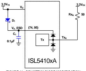
FIGURE 11. SCHOTTKY DIODE MODIFICATION
