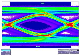
FIGURE 9. ISL54100 EYE DIAGRAM AFTER 15m CABLE
