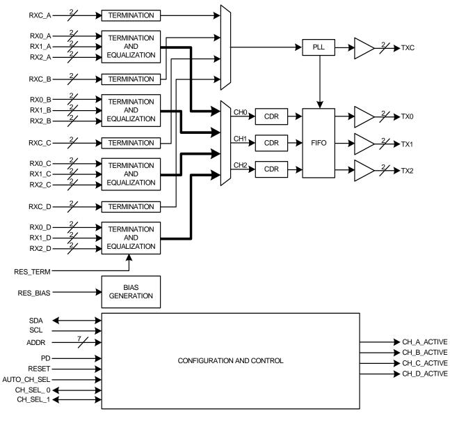
Block Diagram of ISL54100A (ISL54101A, ISL54102A identical except for number of channels)
