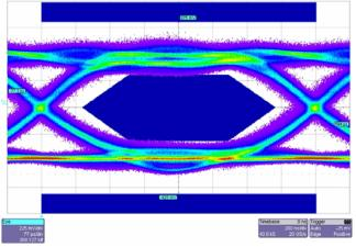
FIGURE 5. EYE DIAGRAM AT OUTPUT OF CHROMA GENERATOR
