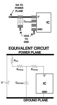
FIGURE 13. OPTIMAL ("T") BYPASS CAPACITOR LAYOUT
