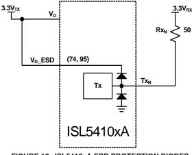
FIGURE 10. ISL5410xA ESD PROTECTION DIODES
