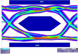
FIGURE 8. EYE DIAGRAM AT OUTPUT OF ISL54100
