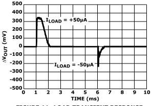
FIGURE 11. LOAD TRANSIENT RESPONSE
