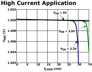
FIGURE 35. DIFFERENT  $V_{\mbox{IN}}$  AT ROOM TEMPERATURE
