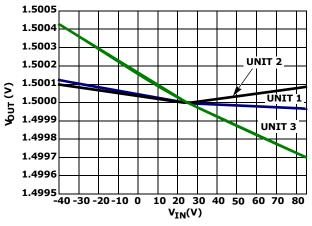
FIGURE 18. V<sub>OUT</sub> vs TEMPERATURE NORMALIZED to +25°C
