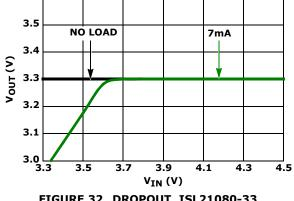
FIGURE 32. DROPOUT, ISL21080-33
