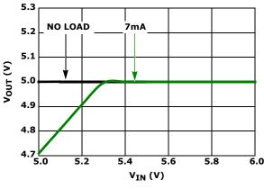
FIGURE 34. DROPOUT, ISL21080-50
