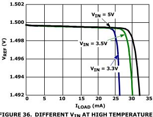
FIGURE 36. DIFFERENT V<sub>IN</sub> AT HIGH TEMPERATURE (+85°C)
