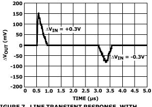
FIGURE 7. LINE TRANSIENT RESPONSE, WITH **CAPACITIVE LOAD**
