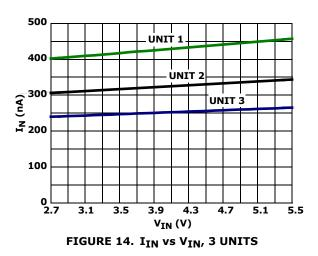
$V_{OUT}$  = 1.5V,  $V_{IN}$  = 3.0V,  $I_{OUT}$  = 0mA,  $T_A$  = +25°C unless otherwise specified.
