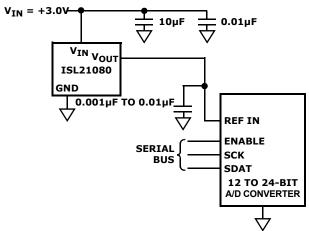
FIGURE 37. REFERENCE INPUT FOR ADC CONVERTER
