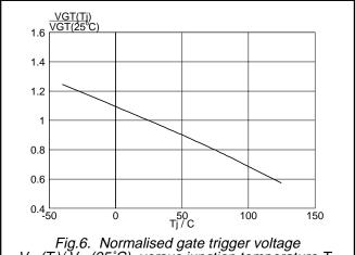
Fig.6. Normalised gate trigger voltage  $V_{GT}(T_j)/V_{GT}(25^{\circ}C)$ , versus junction temperature  $T_{j^{\circ}}$
