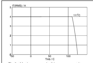
Fig.3. Maximum permissible rms current I<sub>T(RMS)</sub>, versus mounting base temperature  $T_{mb}$ .
