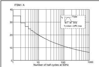
Fig.4. Maximum permissible non-repetitive peak on-state current I<sub>TSM</sub>, versus number of cycles, for sinusoidal currents, f = 50 Hz.
