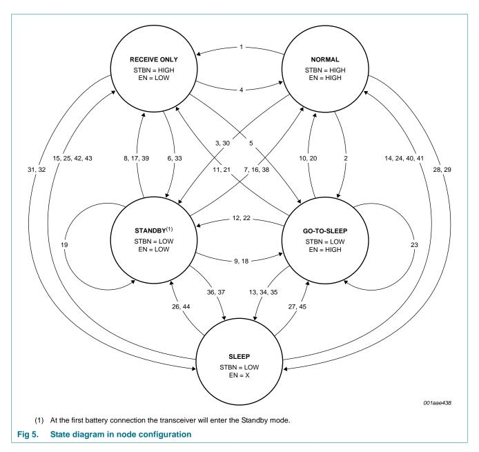
The state transitions are represented with numbers, which correspond with the numbers in column 3 of <u>Table 4</u> to <u>Table 7</u>.
