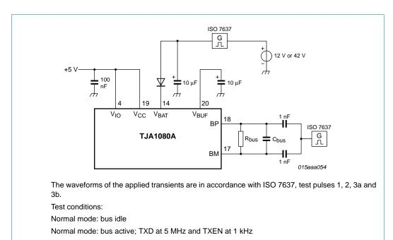
Fig 15. Test circuit for automotive transients
