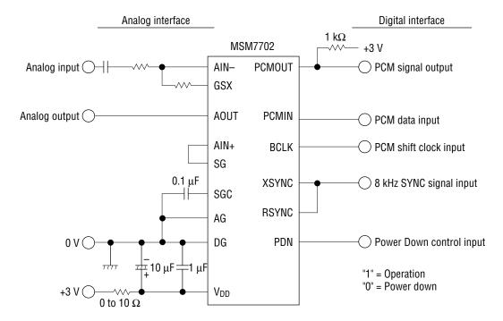
The analog output signal has a maximum amplitude of  $\pm 1.0\,\mathrm{V}$  above and below the offset voltage level of  $V_{DD}/2$ .
