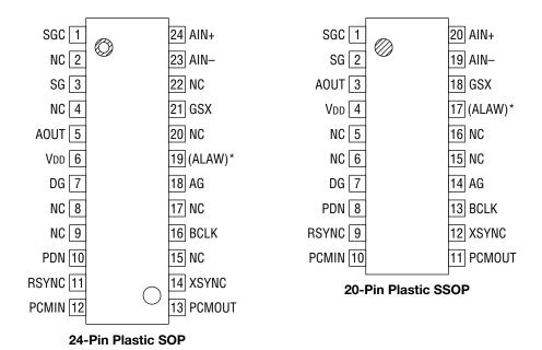
\* The ALAW pin is only applied to the MSM7702-01GS-K/MSM7702-01MS-K.  $\operatorname{NC}$  : No connect pin
