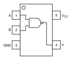
Figure 1. Pinout (Top View)
