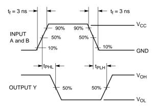
Figure 3. Switching Waveform
