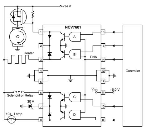
**Figure 1. Typical Driver Applications**
