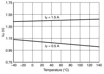
Figure 6. Typical Clamp Diode Forward Voltage
