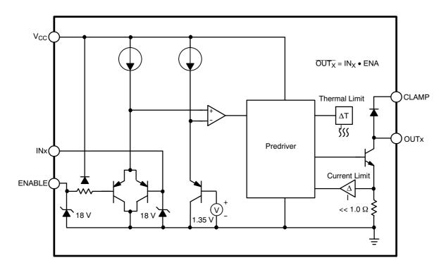
Figure 2. Simplified Block Diagram – Each Driver
