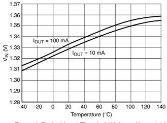
Figure 9. Typical Input Threshold Voltage, V<sub>CC</sub> = 5.0 V
