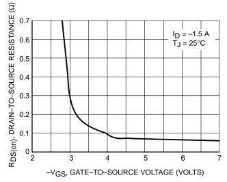
Figure 4. On-Resistance vs. Gate-to-Source Voltage
