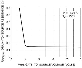
Figure 3. On-Resistance vs. Gate-to-Source Voltage
