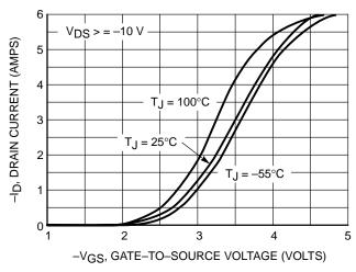
Figure 2. Transfer Characteristics
