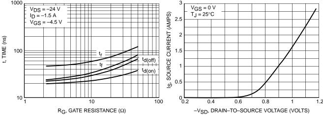
Figure 11. Resistive Switching Time Variation vs. Gate Resistance
