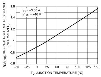
Figure 6. On Resistance Variation with **Temperature**
