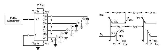
Figure 2. Switching Time Test Circuit and Waveforms
