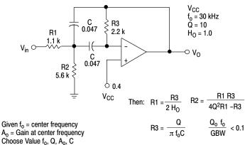
For less than 10% error for operational amplifier, where fo and GBW are expressed in Hz.
