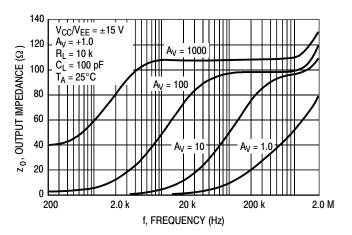
Figure 8. Output Impedance and Frequency
