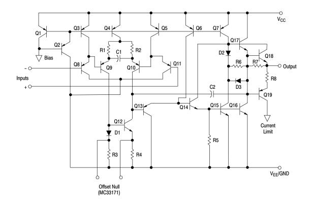
Figure 1. Representative Schematic Diagram (Each Amplifier)
