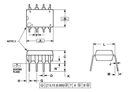
NOTES: 1. DIMENSION L TO CENTER OF LEAD WHEN FORMED PARALLEL. 2. PACKAGE CONTOUR OPTIONAL (ROUND OR SQUARE CORNERS). 3. DIMENSIONING AND TOLERANCING PER ANSI Y14.5M, 1982.
