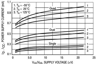
Figure 9. Supply Current versus Supply Voltage
