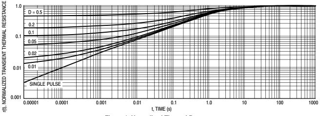
Figure 1. Normalized Thermal Response
