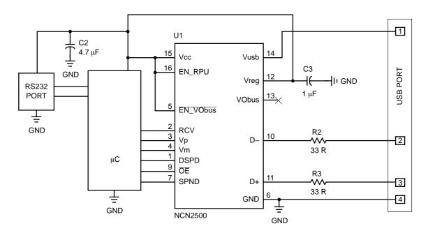
Figure 11. Peripheral are Powered by the Vreg Supply
