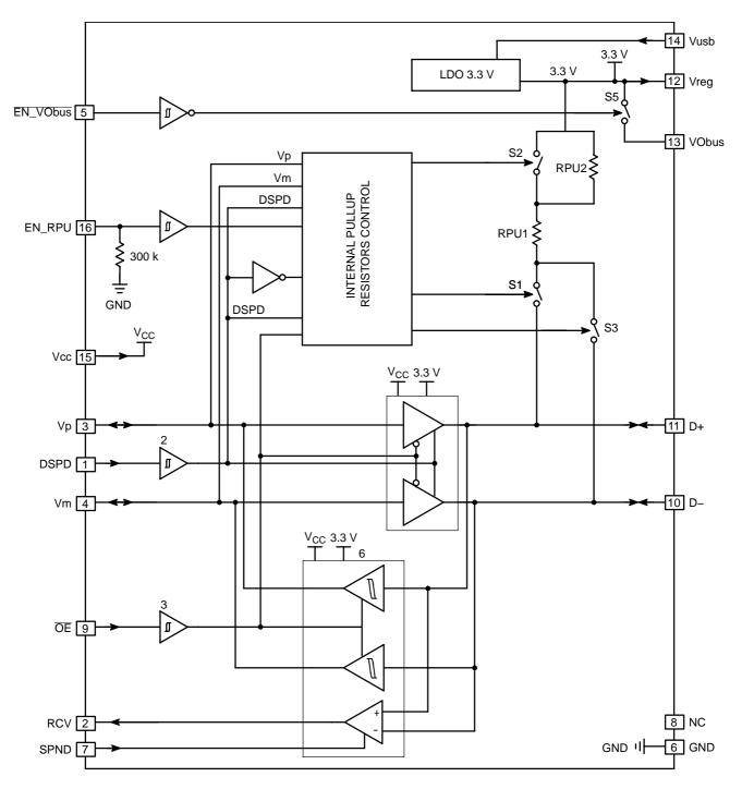
Figure 2. Block Diagram
