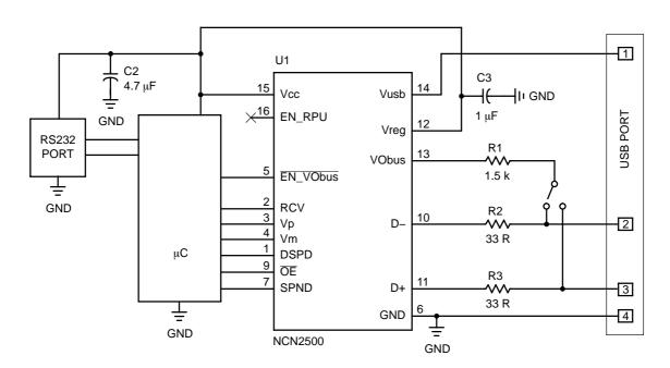
Note: Pin 16 can be left open, due to the internal pull-down resistor, or connected to ground.
