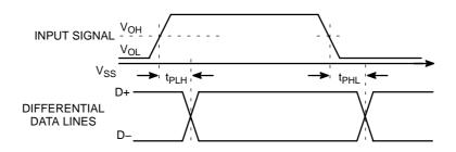
Figure 6. Driver Propagation Delays
