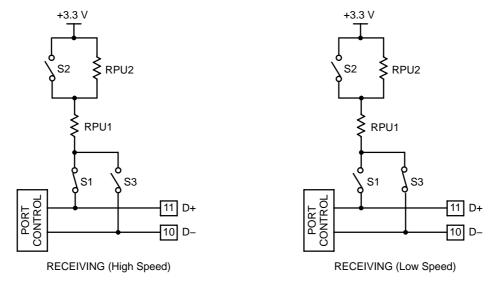
NOTE: Internal Pullup Resistor Range: RPU1: 900  $\Omega$  min–1575  $\Omega$  max, RPU2: 525  $\Omega$  min–1515  $\Omega$  max
