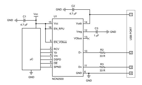
In this application, the two internal pullup resistors (RPU1 and RPU2) are used to bias the USB line. Consequently, the VObus voltage is deactivated (Pin 5 connected to Vcc).
