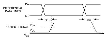
Figure 5. Receiver Propagation Delays
