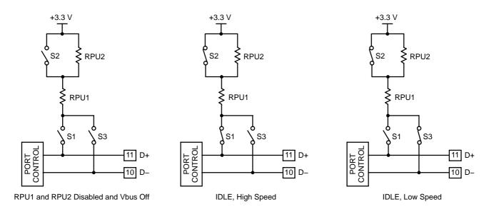
Figure 8. Internal RPU1 and RPU2 Pullup Resistors Operation, IDLE Mode
