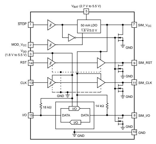
Figure 3. NCN4555 Block Diagram
