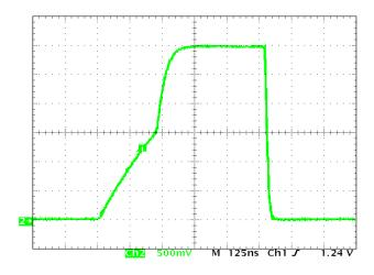
Figure 10. SIM\_IO Typical Rise and Fall Times with Stray Capacitance > 30 pF (33 pF Capacitor Connected on the Board)
