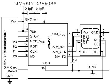
Figure 1. Typical Interface Application
