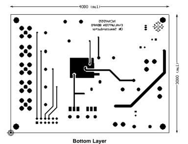
Figure 13. NCN4555 Printed Circuit Board Layout (Engineering board)
