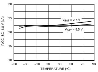
Figure 7. IV<sub>BAT</sub> vs Temperature at 1.8 V
