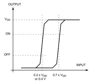
Figure 11. Typical Schmitt Trigger Characteristics
