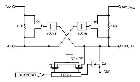
Figure 9. Basic I/O Line Interface
