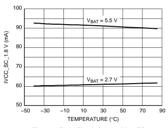
Figure 4. Short Circuit Current IV $_{CC}$ SC vs Temperature at SIM $_{VCC}$  = 1.8 V (MOD $_{VCC}$  = LOW)
