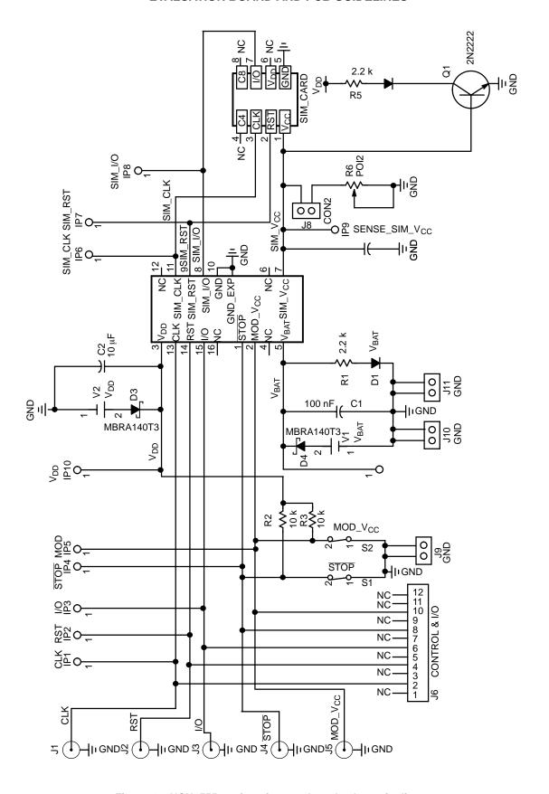
Figure 12. NCN4555 engineering test board schematic diagram
