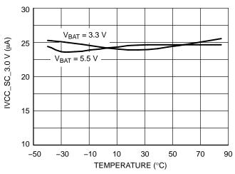
Figure 6. I<sub>BAT</sub> vs temperature at 3.0 V
