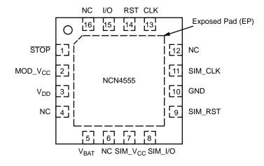
Figure 2. QFN-16 Pinout (Top View)
