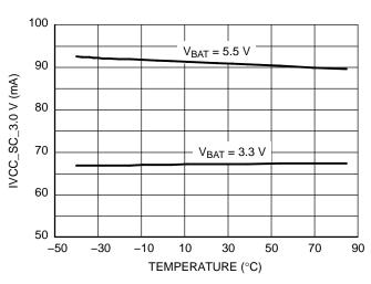
Figure 5. Short Circuit Current IV $_{CC}$ SC vs Temperature at SIM $_{CC}$  = 3.0 V (MOD $_{CC}$  = HIGH)
