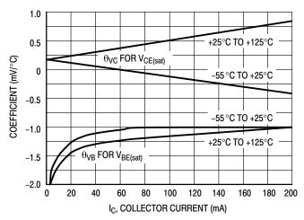
Figure 17. Temperature Coefficients
