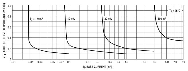
Figure 15. Collector Saturation Region
